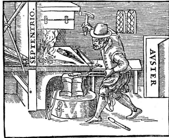
Fig. 1. Diagram from Gilbert's De Magnete , 1600 — forming a magnet by hammering a piece of iron in the earth's magnetic field.
