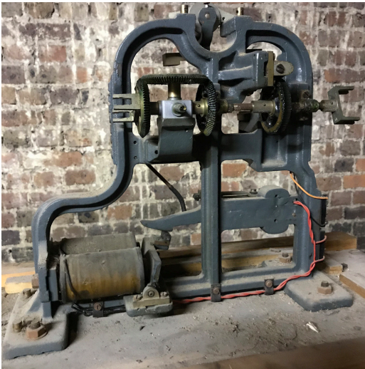
Fig. 6. The sad remains of the Gent 'waiting train' movement. The Meccano 'windmill' arrangement (see text) was fixed to a further wheel in the nest of bevels. Each quarter an arm closed a micro-switch in front of the main drive coil armature, releasing the chiming train of the flatbed. Photo Robert Wren.
