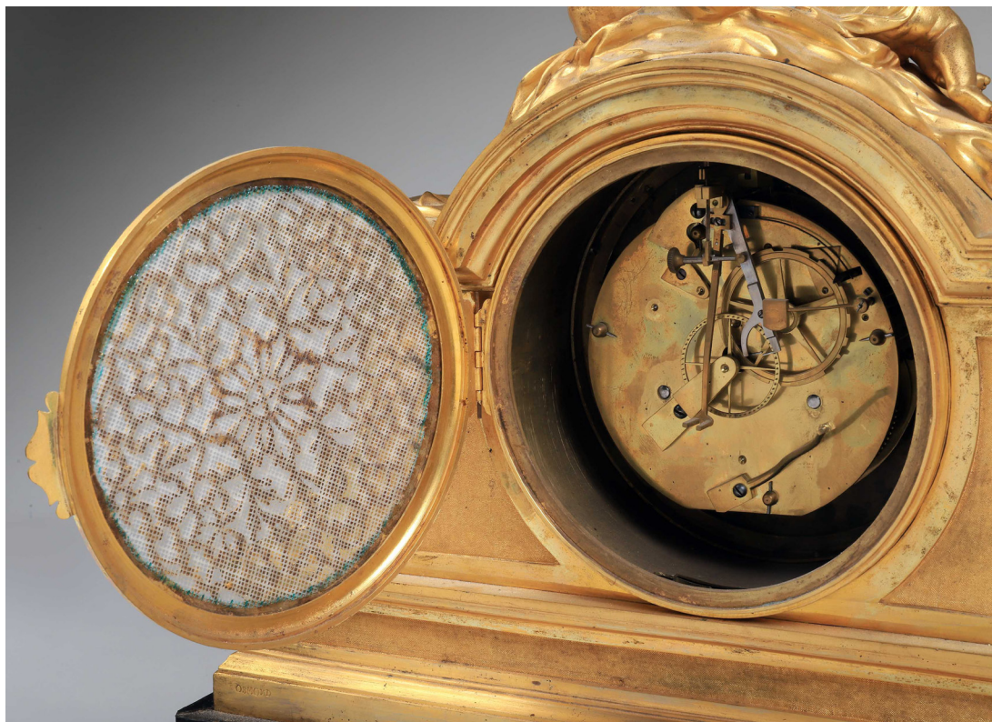
Fig. 4. Backplate with bell removed to show the escapement.
