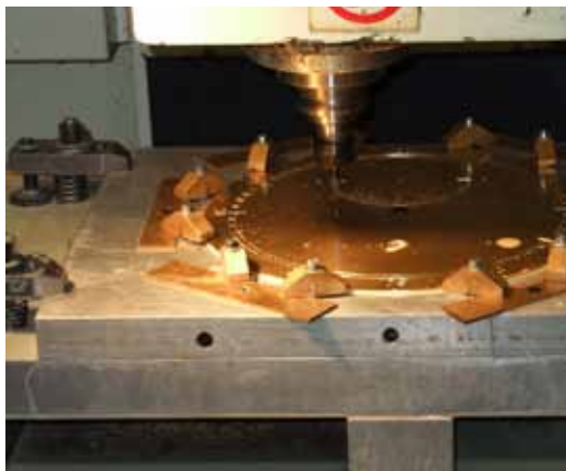
The Erwin Sattler works: machining a regulator dial. Photo Mike Wilson.
