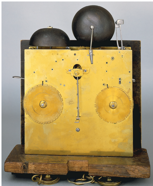
Fig. 33. Rear view of the movement of an Edward East petite-sonnerie longcase clock, c. 1675. Image courtesy of Dr John C. Taylor.
