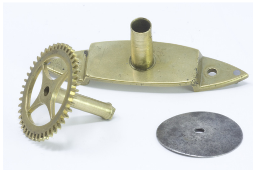
Fig. 20. Characteristic lozenge-shaped hour bridge, with bevelled edges, from the same Aylward clock.
