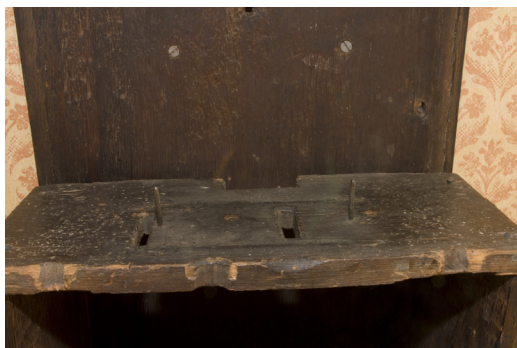
Fig. 24. Spikes on the seat board of the Aylward clock, which prevent movement during winding.
