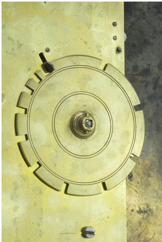
Fig. 14. Count wheel from a longcase signed John Aylward of Guildford, c. 1695.
