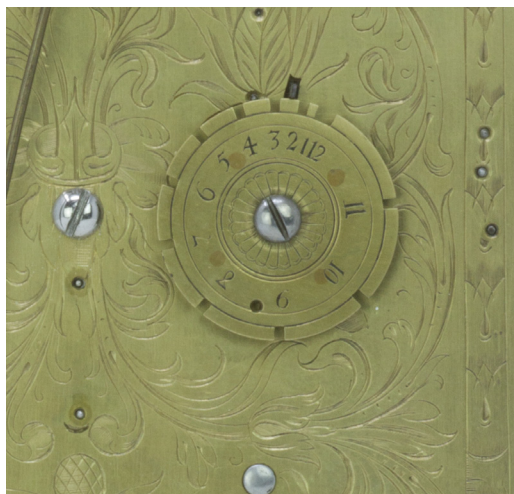
Fig. 9. Count-wheel from the same Burgis clock.
