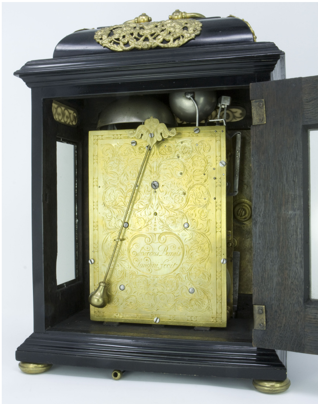
Fig. 6. Rear plate of a spring-clock, signed Edward Burgis, c. 1695-1700, with pull-repeating.
