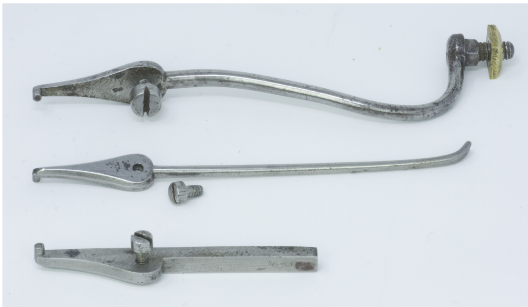
Fig. 22. Bell-stand, hammer spring and hammer stop, from the Aylward clock in Fig. 14.
