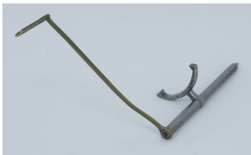
Fig. 19. Pallets and brass crutch, from the Aylward clock in Fig. 14.
