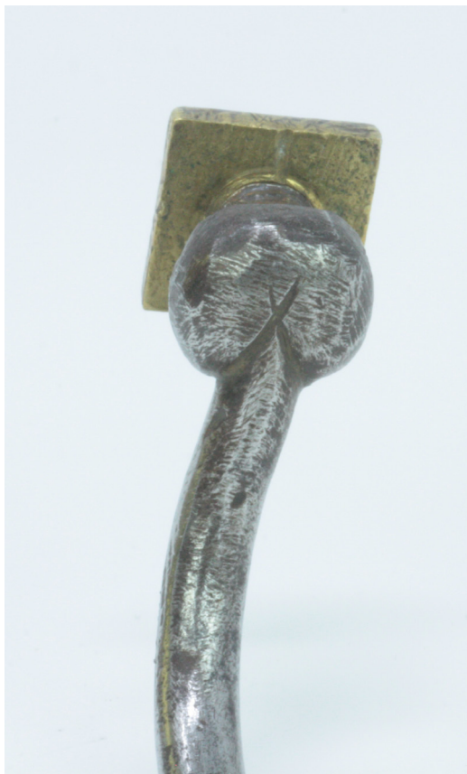
Fig. 23. The distinctive domed shoulder on the bell-stand of the same Aylward clock.
