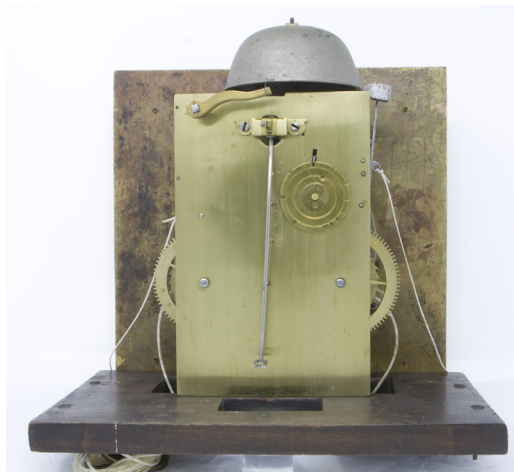
Fig. 29. The rear plate of the Burgis clock in Fig. 3, showing the relatively high position of the barrels in the plates.
