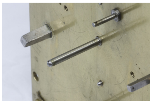
Fig. 21. Parallel-profiled centre arbor, longcase clock re-signed Seignior, as in Fig. 17. Photo: James Nye (© Harris (Belmont) Charity).
