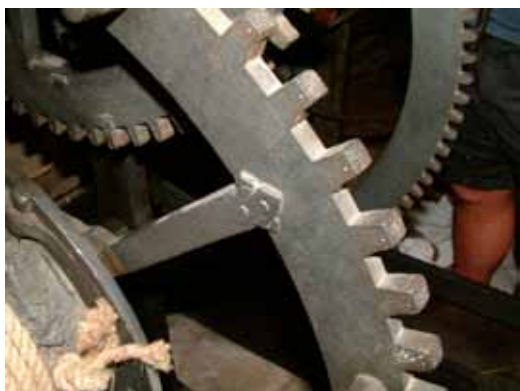
Fig. 10. Details of tooth forms, left to right Salisbury, Wells and (above right) Rye.
