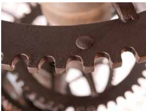
Fig. 10. Details of tooth forms, left to right Salisbury, Wells and (above right) Rye.
