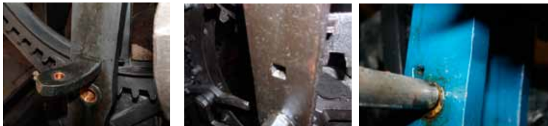
Fig. 15. Evidence of the fixing of the bottom cocks for the verge and foliot escapement, left to right Salisbury, Wells and Rye; the Salisbury clock shows a replacement by Smiths of Derby (1959). In all three clocks, the cock was positioned just above the second arbor of the going train.
