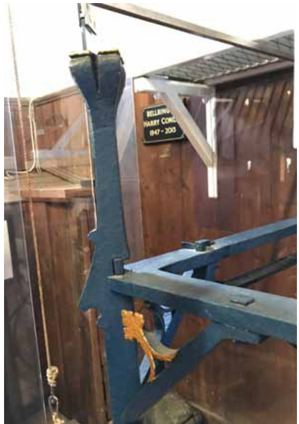
Fig. 19. Rye top corner detail. This shows a different construction from Salisbury and Wells, often found in chamber clocks, but arguably insufficiently robust for a turret clock.
