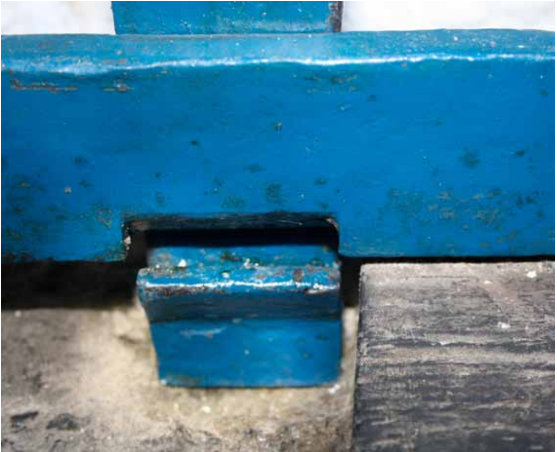
Fig. 23. Rye front train bar (going and striking) detail. A type of joint more often found in chamber clocks, which, though beautifully crafted, allows for movement of the train bar once in position. It lacks necessary rigidity, and suggests an earlier date, not later.
