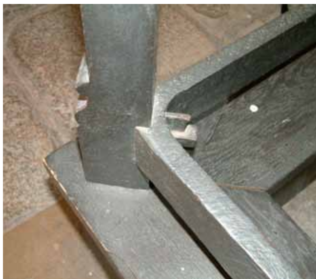
Fig. 17. The bottom section of the construction of the frame (Salisbury) showing the detail of the mortice and tenon, and the recessing into the upright corner post by the bottom rectangular frame. All three clocks exhibit the same construction. This construction, along with the interlocking train bars, confers two advantages. The particular combination of horizontal and vertical elements in the frames of the clock confer excellent strength. Further, the method by which the train bars support the rectangular frames shows an understanding of the forces applied to the clock by the driving weights, making it very strong and stable. The method of construction also allows for greater ease in initial transport from the place of manufacture, and then lifting in parts to the relevant position within the tower.
