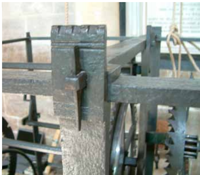
Fig. 21. Top train bar fixing. The same construction is used in all three clocks. It gives strength and support to the main frame.
