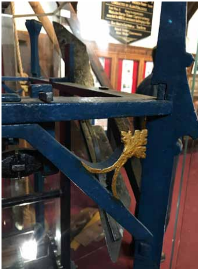
Fig. 20. Rye corner braces. These appear to be later additions to strengthen the inherently weaker top joints, necessitated by the addition of the quarter-striking train, suspended to the side of the main frame, the weight for which imposes a strain on the whole construction.
