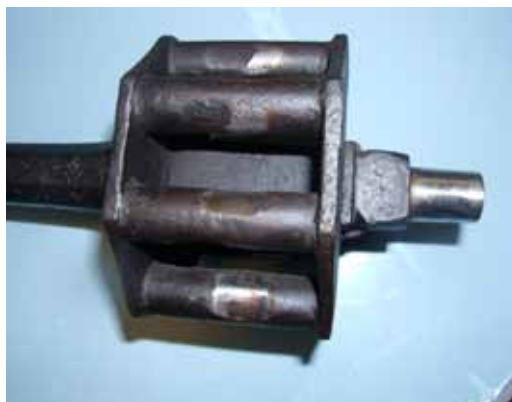
Fig. 9. Details of pinions, left to right Salisbury, Wells and (below left) Rye.
