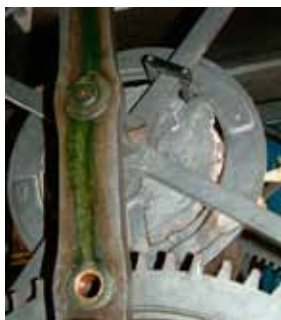
Fig. 11. Winding barrel click work, left to right Salisbury, Wells and Rye.
