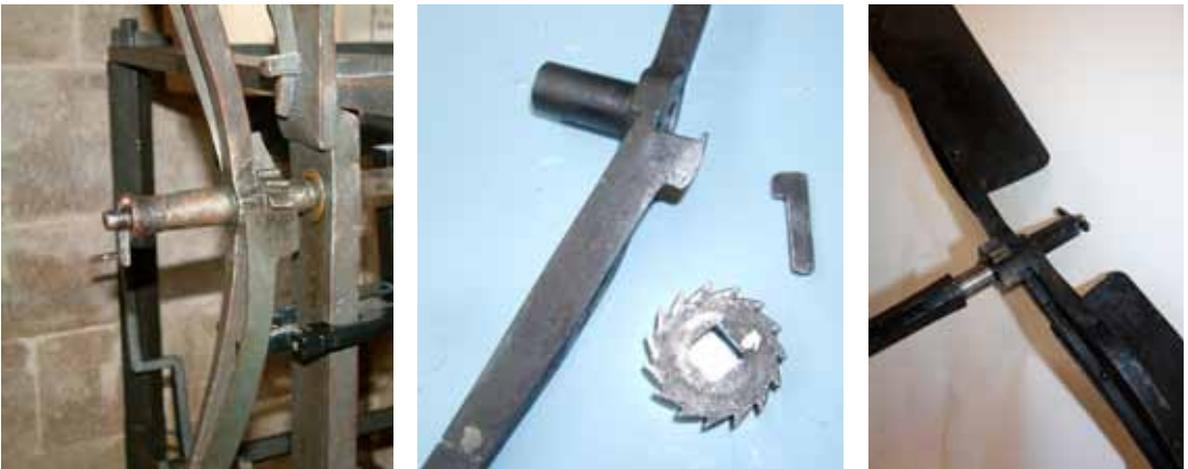
Fig. 8. Fly fans and ratchets, left to right Salisbury, Wells and Rye.
