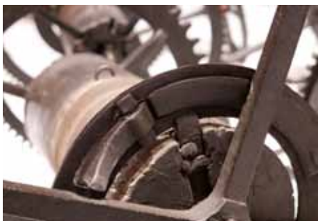
Fig. 11. Winding barrel click work, left to right Salisbury, Wells and Rye.
