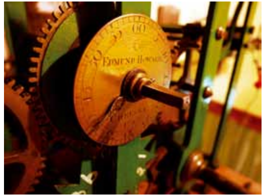
Fig. 12. Setting dial of the Gautby Old Hall clock. Image courtesy of Keith Scobie-Youngs.
