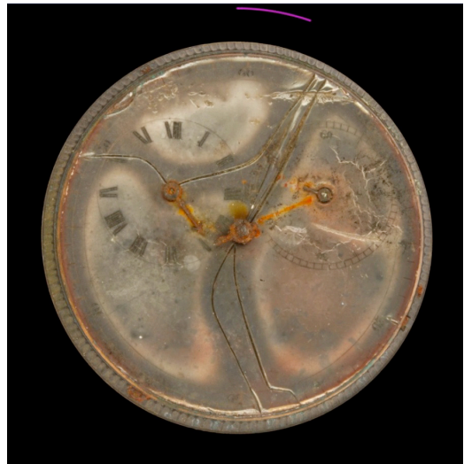
Figs 8, 9 and 10. Chronometer No. 8 by Johann Heinrich Seyffert: damaged original and virtual reconstruction of the dial and the movement.
