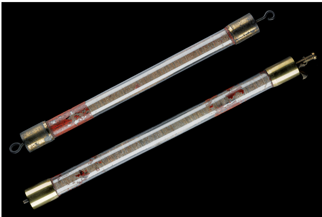
Fig. 1. Ronalds' dry piles, manufactured by Singer (1814). Source: Science Museum, reproduced with permission.
