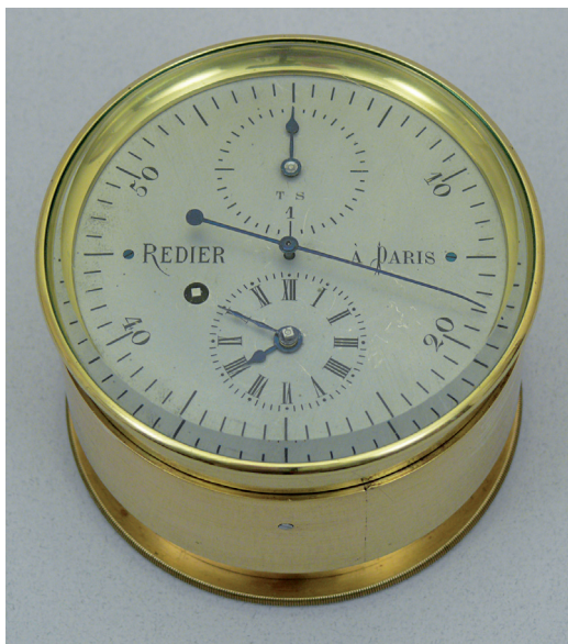
Fig. 6. Redier's Comparateur Chronométrique . It contains two movements (one in the base and one beneath the dial) that can be rotated relative to each other by turning their outer casings, thereby altering the time shown by the hands. Diameter 90 mm.
