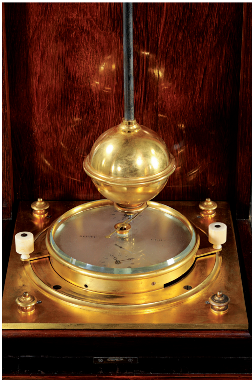
Fig. 4. The dial of the pendule conique and the two movements (primary and secondary) mounted beneath it form a single assembly that can be rotated relative to the pendulum. The rotating arm above the dial maintains the pendulum in motion and is driven by the primary movement. © Musée des arts et métiers-Cnam, Paris / Photo Michèle Favareille.
