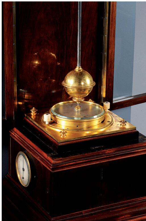
Fig. 5. The dial on the side of the case shows the alteration, in hundredths of a second, made to the time shown by the hands of the pendule conique when the mechanism is rotated. © Musée des arts et métiers-Cnam, Paris / Photo Michèle Favareille.
