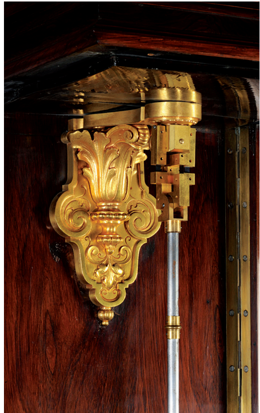
Fig. 2 (left). Redier's Comparateur à Pendule Conique, 1859. This conical pendulum clock has a mechanism that can be rotated about the axis of the pendulum, thereby altering the time shown by the hands. Fig. 3 shows the suspension in the pendule conique that enables the pendulum to follow a circular path. © Musée des arts et métiers-Cnam, Paris / Photos Michèle Favareille.
