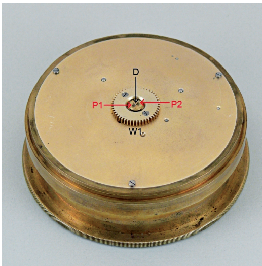
Fig. 8. The upper plate of the primary movement. The disc D , carrying the pins P1 and P2 , is mounted on the escape wheel arbor. The pins lock the arm A of the secondary movement shown in Fig. 9 and the wheel W1 engages with W2 .
