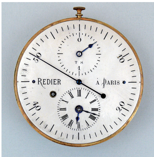
Fig. 10. The dial of the comparateur . The indicator in the top half of the dial registers the relative rotation of the movements. It indicates here that the seconds hand has been advanced by three tenths of a second.
